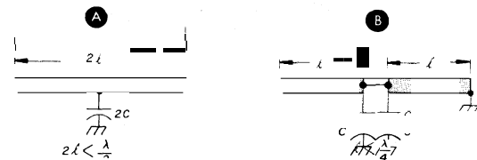
fig. 2. Capacitively loaded half-wavelength stripline resonator (A), and equivalent circuit using two quarter-wavelength lines (B). A groundplane is assumed to be present in both cases.
