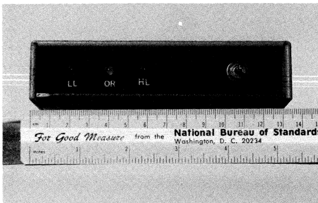
Front view of the VFO-stabilizing unit. The three LEDs are used to indicate the position of the control voltage within its total range.
