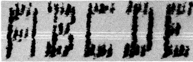
Hell writing. This enlargement shows how each character takes the space of seven image lines. As a result of the relatively slow-moving tape, the characters hang slightly over.
