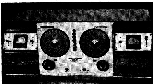
fig. 5. A Hallicrafters dual-diversity receiver, Model DD-1. This is the only commercially made receiver intended for diversity reception, circa 1939.
