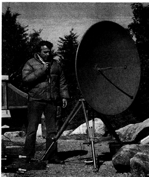
10-GHz Gunnplexer system setup by the W1FC group on Pack Monadnock in New Hampshire during the September vhf/uhf contest. Two-way communications were established with Gunnplexer-equipped stations in Maine, New Hampshire, and Vermont.
