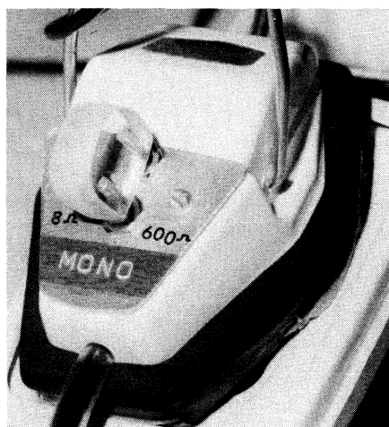
The switching arrangement is shown in this view of the dual-impedance headphones. Photo by WD9CXG.
