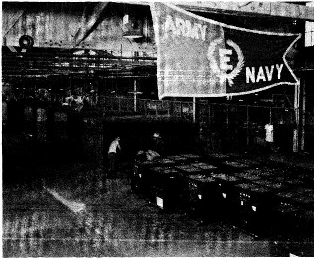
Hallicrafters won five Army-Navy E awards during World War II for excellence in production. This photo shows BC-610 transmitters in final inspection before they were mounted in the communications vans in the background.
