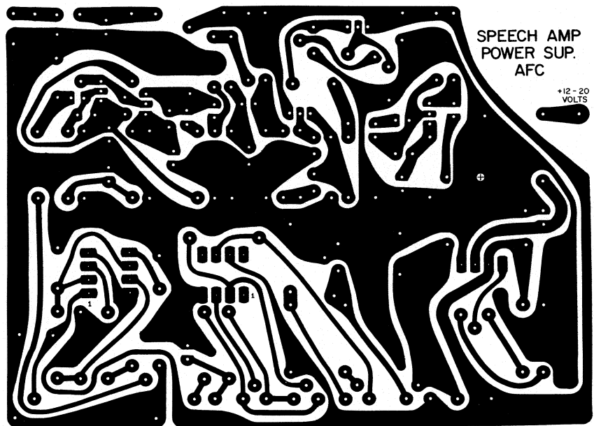
fig. 23. Full-size printed-circuit layout for the Gunnplexer speech amplifier, tone oscillator, AFC amplifier, and voltage regulator. Component layout is shown in fig. 22.
