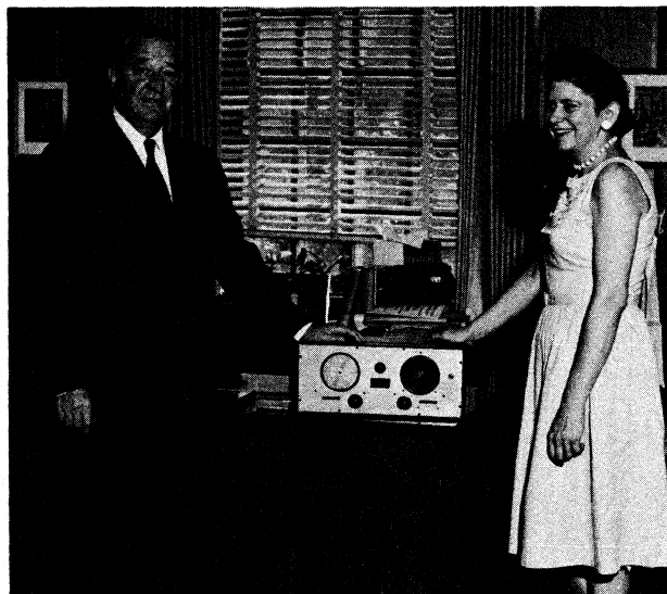
Bill Halligan and wife, Katie, with the very first model Sky Rider receiver of long ago. Receiver was a trf job, soon to be supplanted by the Super Skyrider. a superheterodyne.
