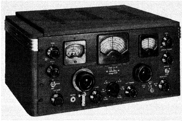
The famous Hallicrafters SX-28 receiver. Over 50,000 were produced for the Allied Forces. High styling and good performance made the receiver a favorite among pre-war Amateurs. Receiver incorporated two rf stages and tuned up to 43 MHz. In 1946 it was replaced by the SX-42.
